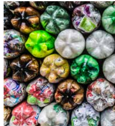
» Figure 2: Ecobricks made using plastic waste
