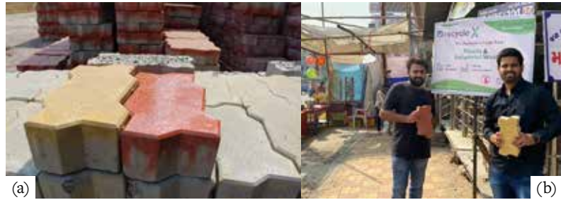
» Figure 1: Building materials from various wastes (a) paving bricks made of plastic and industrial waste (b) pavement made from waste-based paving bricks
